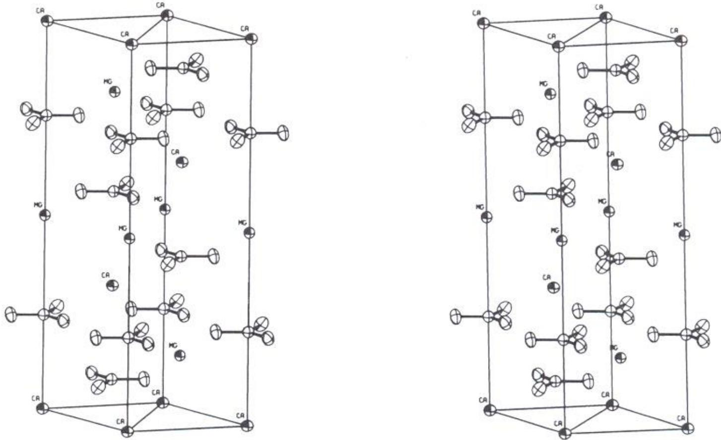
Figure 20. Stereoscopic projection of the hexagonal unit cell for dolomite ( $a = 4.81 \text{ \AA}$ ,  $c = 16.00 \text{ \AA}$ ), prepared using the program ORTEP (Johnson, 1965).  $c$  is vertical; compare with Figure 4 for the disposition of axes. Cation layers occur at intervals of  $1/6 c$ ; carbonate layers at levels  $\pm z_0$ ,  $1/3 \pm z_0$ ,  $2/3 \pm z_0$ .
