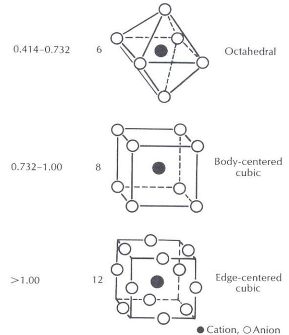
**Figure 7.4** Possible arrangements of ions in crystals for limiting values of the radius ratios and different values of the coordination number.
