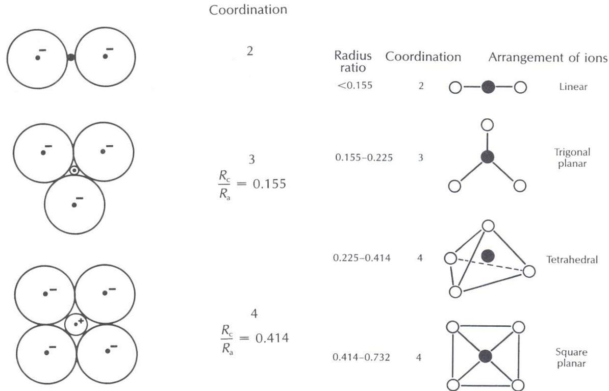
**Figure 7.2** Examples of closest packing of anions around cations at increasing values of the radius ratio. When  $R_c/R_a > 0.155$ , three anions fit around the cation and when  $R_c/R_a > 0.414$ , fourfold coordination occurs. Coordination numbers 6, 8, and 12 are also important in mineral structures and are pictured in Figure 7.4.
